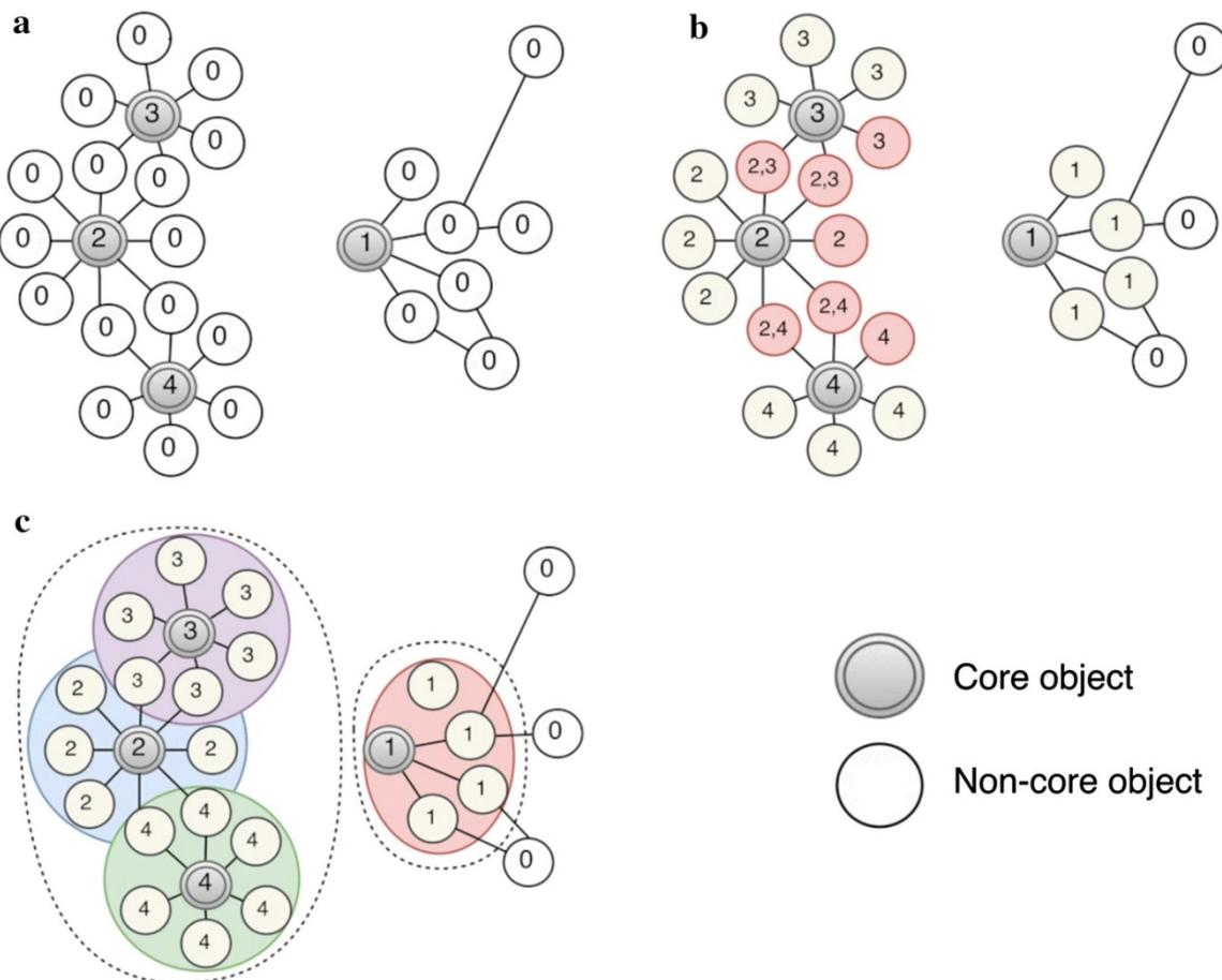
**Figure 15:** Graphic representation of the clustering approach. *i)* Initialization of cluster identifiers *ii)* Core objects propagate their cluster ID to their neighbours. Nodes highlighted in red receive multiple messages. *iii)* Multiple cluster IDs received by the same node are aggregated. Dotted lines represent the final clustering result, after some iterations [9].
