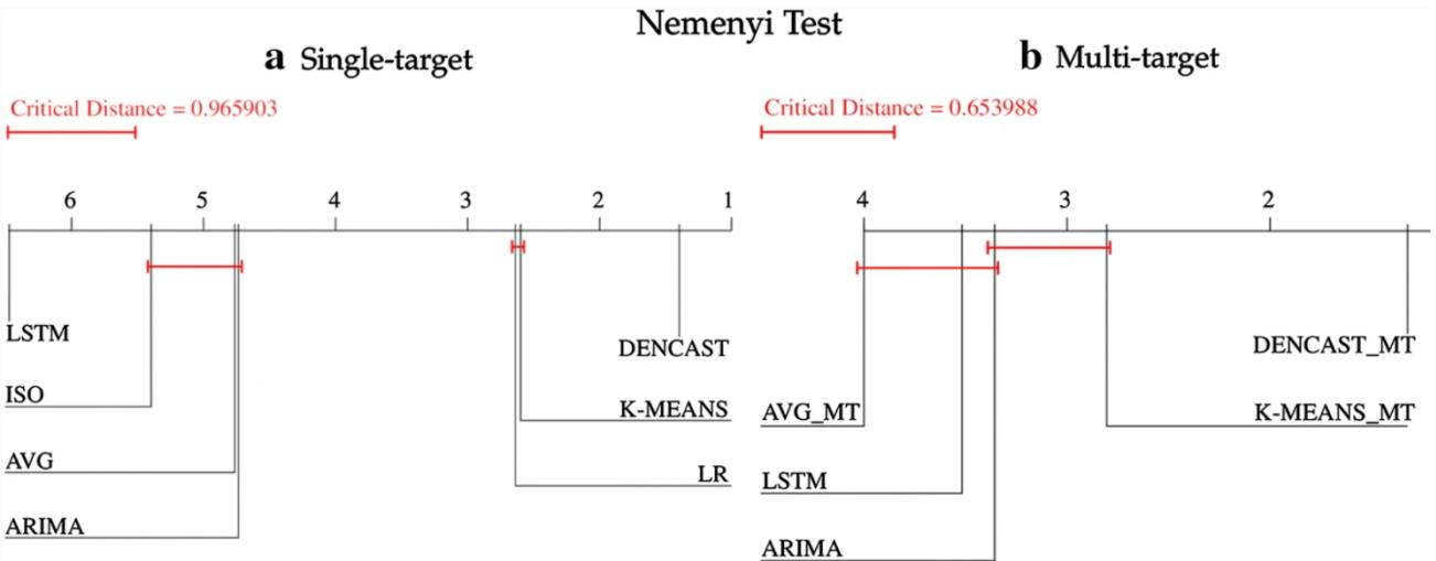
**Figure 16:** Nemenyi test for a single-target and b multi-target settings. If the distance between methods is less than the critical distance (at  $p\text{-value} = 0.05$ ), there is no statistically significant difference between them.
