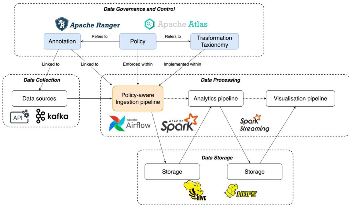
**Figure 6:** Technologies and frameworks in data ingestion and access control.
