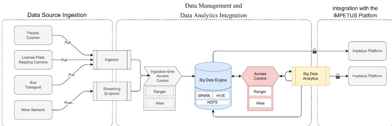
Figure 31: Data management and data analytics integration – Mapping to the Engine
