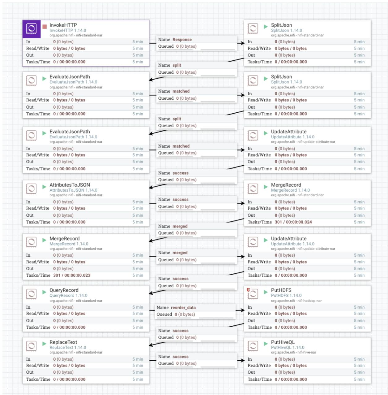
Figure 24: Ingestion flow using NiFi.
