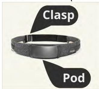
The Muse S integrates EEG and PPG sensors in one, wireless headband. The clasp can be used to adjust the band to fit snugly on your head. The “Pod” houses the main sensors, electronics and battery. Additional sensors are the gold metallic strips on either side of the head, resting on the ears.
