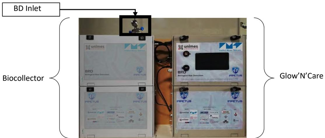
**Figure 17: Identifying biocollector and Glow'N'Care device**
